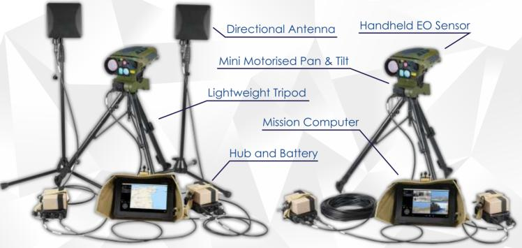
NOTE: A system can be formed of both wired and wireless interconnects
